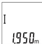
Briefly press the measuring button **2** to initiate the measurement. The current measured value **c** appears in the bottom line of the display. The laser beam is switched off.
