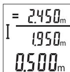
To switch on the laser beam briefly press the measuring button **2**. To switch on the laser beam briefly press the measuring button **2** again. The current measured value **c** is displayed in the bottom line. The previous measured value **b** is displayed in the middle line. In the top line the auto-sum **a** (the sum of the current and previous measured value) is displayed.
